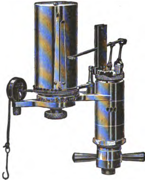
FIG. 228.—A Typical Steam Engine Indicator. It consists of a cylinder, shown at the right, within which works a piston under tension of a helical spring of predetermined strength. The rod attached to the piston carries a pivoted arm which works on the horizontal lever, shown at the top of the cylinder. This lever carries a pencil bearing against the rotatable drum, shown at the left. This drum is so arranged with a spring that it may be rotated by the pull on the attached string. A sheet of paper is wound on the drum and held in place by the spring clips. The steam pressure in the cylinder acting on the spring enables the pencil to mark; the indicator card being traced by the rotative movement of the paper drum.
